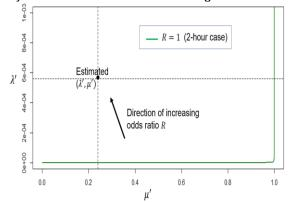
Note: The lines plot values of cloud incident rate  $\lambda'$  and cloud repair rate  $\mu'$ , expressed as per-hour quantities, for which systemic events have the same probability in the no-cloud baseline and the cloud scenario, given the parameter estimates for  $\lambda$  and  $\mu$  based on CCP outage data. A systemic event occurs whenever the same 3 firms are out simultaneously for at least 2 hours. The y-axis is truncated at  $\lambda' = 0.1\%$  for clarity.
