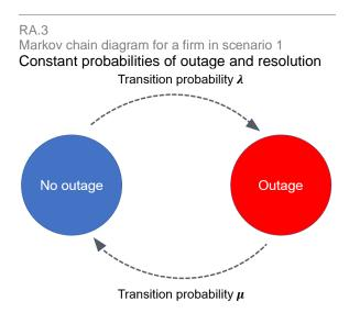
Note: Markov chain diagram for a single firm in the no-cloud baseline scenario, in which possible states of the firm are represented by coloured circles.
