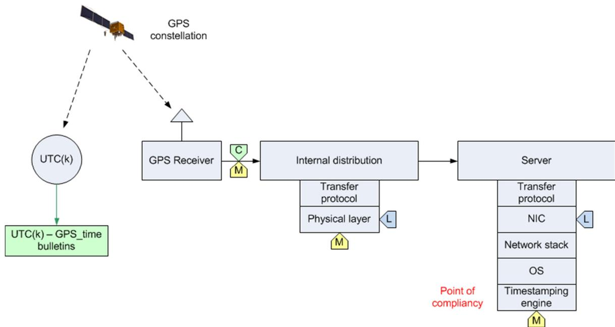
Figure 3: Diagram of a typical GPS-based distribution, indicating the traceability chain. 'C' indicates the point where a calibration may be carried out to determine the offset introduced by the GPS receiver, 'L' indicates points where latency (distribution offsets) can be determined, and 'M' indicates points where continuous monitoring of the time distribution can be carried out.
